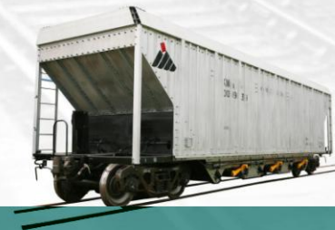
Km98 Type Aluminum Alloy Hopper Wagon for Coal Transportation
